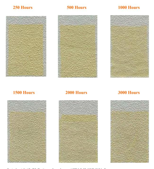
EnviroLastic® AR 425, Testing performed as per ASTM G-53, UVB-313 bulbs
