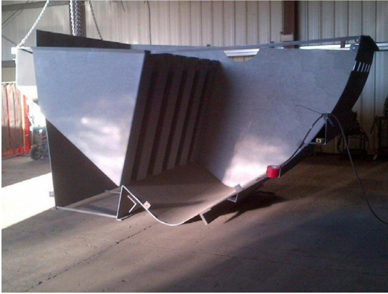
When Spray All Poly, LTD came onsite, they wiped down the material with VersaFlex Dzolv solvent and applied the VF-330 to all the seams.
