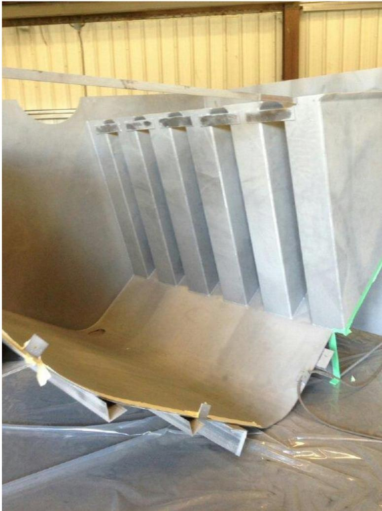
Due to the size, weight and intricate location of the hoppers in the coal plant, the three piece hopper system was pre-sprayed at Fabrite, located in Cranbrook, BC. The parts were extremely intricate and required a great deal of application experience and ingenuity just to spray the parts. The previous “epoxy coating” method called for 20-30 mils of epoxy. Then they would place a plastic insert in place between the epoxy coating and the coal slurry.
