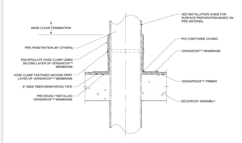
NOTE: IF EXISTING FOAM OR OTHER MATERIAL IS PRESENT AROUND PENETRATION, REMOVE TO FLUSH WITH DECK PRIOR TO PLACEMENT OF VERSAROOF™ PRODUCTS. ENSURE PENETRATION IS STABLE PRIOR TO PLACEMENT
