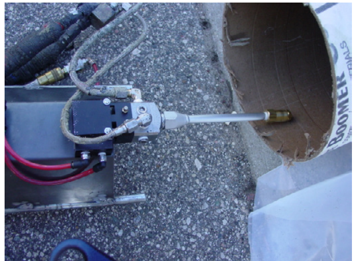
Figure 10: Commercial PUA Pipelining Spray Head, Spinning Cup & Static Mix
