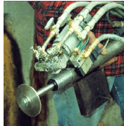
Figure 9: Spray Gun / Spinning Disk for Manhole Lining
